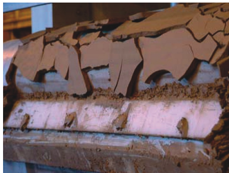
Belt Filter Vacuum System Photo courtesy of Larox
