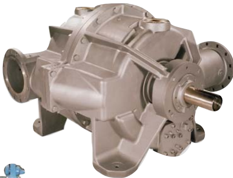
GARO single and two stage Compressors Capacity: 100 to 3,400 m 3 /h Discharge pressure: to 15 bar abs.
