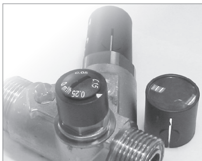
TemCon + The plastic cap is dismantled by means of a screwdriver that fits into the slot in the cap. Hereinafter the manually operated by-pass can be set steplessly to a Kv-value between 0.0 and 0.3.
